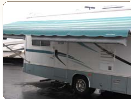
RV AWNING Clip shown here attaching ClimaCover Awning Anchor to Standard RV Awning.
